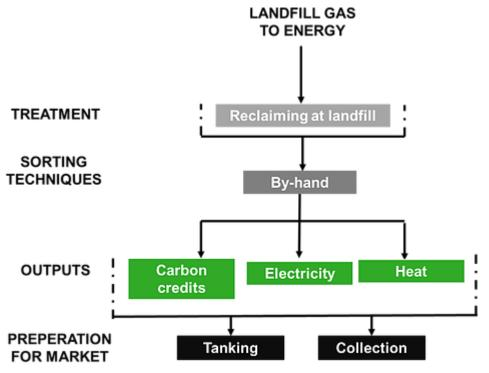
Figure 13-4: Landfill gas to energy process
