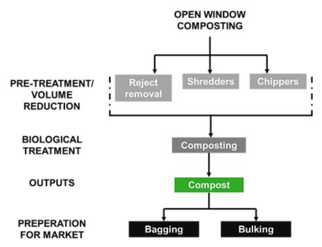
Figure 13-1: Open windrow composting
