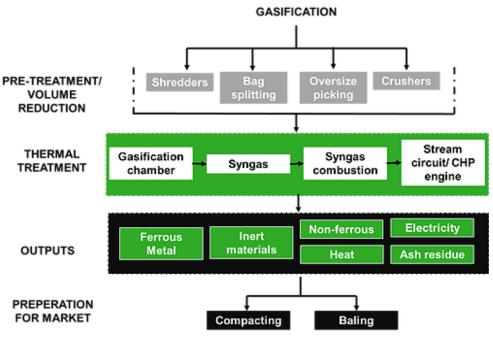
Figure 13-9: Gasification process
