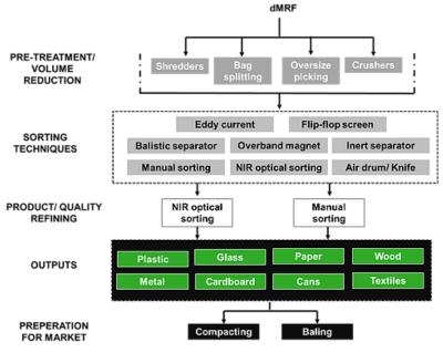
Figure 13-3: dMRF process
