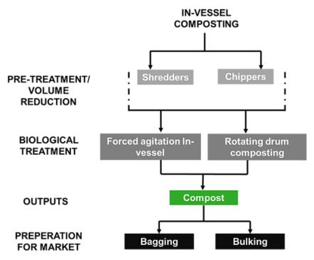
Figure 13-8: In-vessel composting
