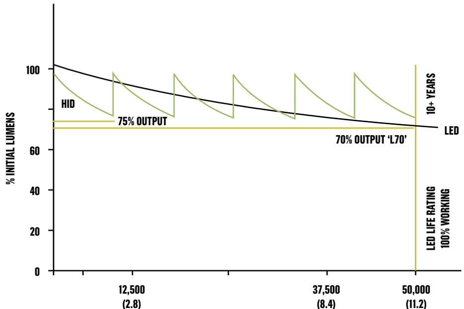
**DIAGRAM:** Comparison of lamp life and lumen maintenance between high intensity discharge (HID) lamps and LEDs. The LED efficiency and lumen maintenance can negate the need to replace multiple HID lamps over the same period.<sup>49</sup>
