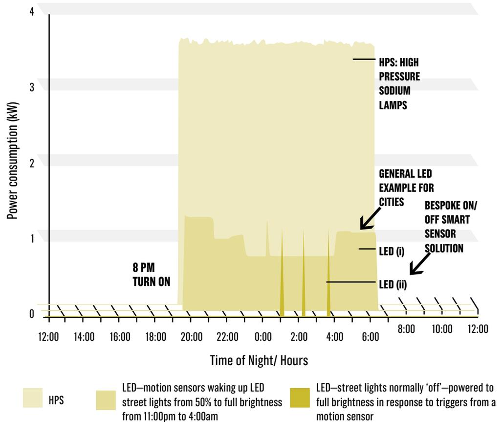
**DIAGRAM:** Comparison of electricity consumption of two street lighting systems (HPS vs LED) over the course of a 24 hour period.
